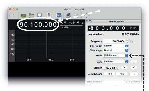
Adjusting the frequency in Gqrx is a little tricky. Click the top half of any digit to tune up, and click the lower half of a digit to tune down. You can also click a digit and type a number on your keyboard to replace it.
