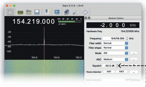
To turn off the audio when there isn't a strong signal, you can adjust the **squelch threshold**. Start at -30 dB and look for a value that lets signals through while silencing the noise.
