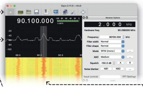
The window with the bouncing white line is called the **spectrum frame**, showing how much energy is present at various points along the RF spectrum. In the example above you can see three large peaks, corresponding to three different FM stations.
