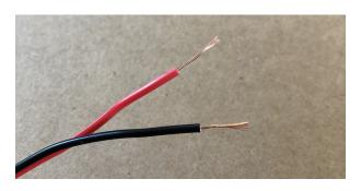
The example project uses red and black wires. The red wire will be the **signal wire**, and the black wire will be the **ground wire**. The signal wire will connect to a GPIO pin on your Pi Pico, and will carry the audio signal to the speaker. The ground wire will connect to a ground pin, letting electricity flow back into the Pi Pico. (It doesn't matter what wire colors you use, but you should decide which is which.)
