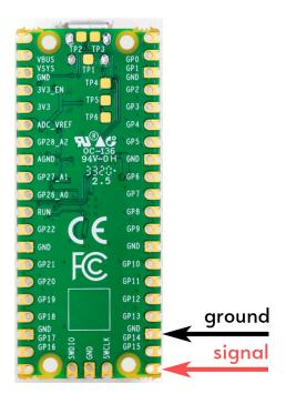
This tutorial uses **GPIO pin 15** for the **audio signal**. If you're looking at the back of your Pi Pico, **GP15** is at the bottom right corner. There's a ground pin two spaces away. (Note that all the ground pins have square outlines, while the rest are round.)
