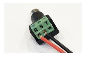
If you're using a stereo audio jack, you can connect the signal wire to the tip(T) terminal to play audio only in the left channel. Or you can connect it to the ring(R) terminal to play through the right channel.
