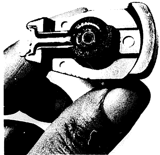
This rotor matches the distributor cap with a bad center contact and will have to be replaced.
