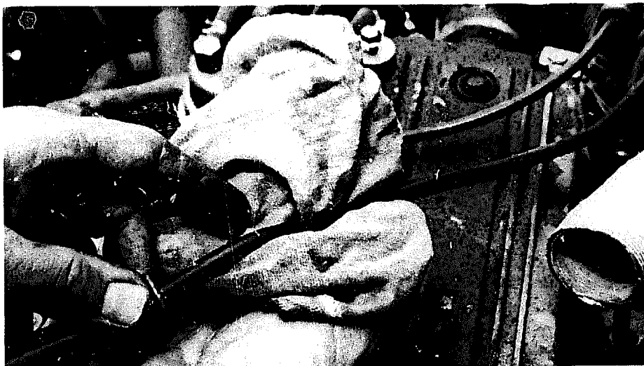
Inspect each wire for burns, cracks and other damage while wiping it clean.
