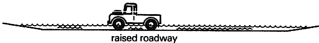
Figure 21(b). Wide crossing, shallow flood.
