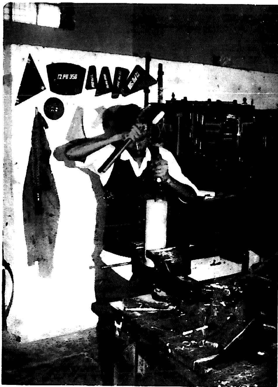
Chiseling the square hole in the crosshead
