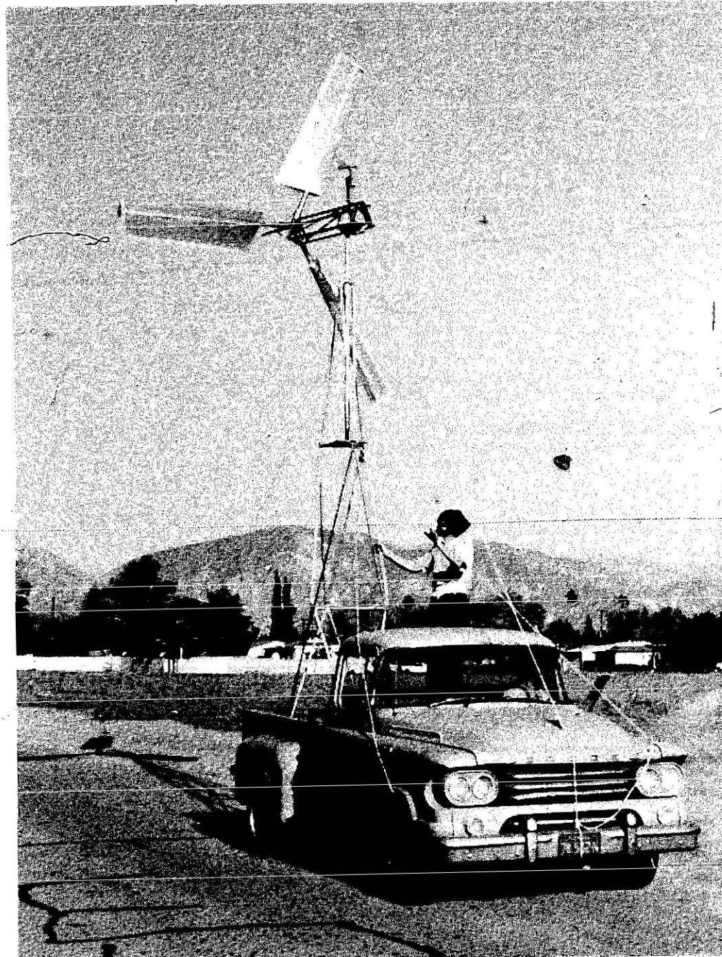
Fiberglass-bladed rotor being tested on the back of a pickup truck. Wind machines are usually tested, often to complete destruction, before final designs are ready.
