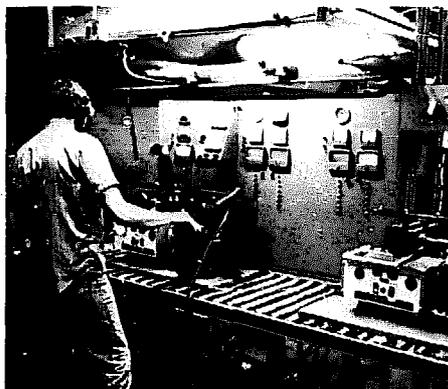
**ENGINE TESTING** is an industrial application in which the Gemini can be used to recover significant amounts of energy which would otherwise be wasted.
