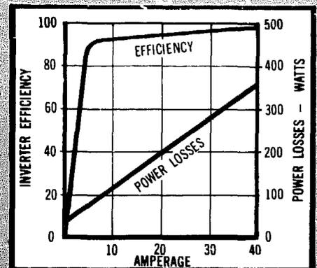
In addition to minimizing system losses associated with current level, operating at higher voltages results in a minimum VAR load imposed on the AC lines.
