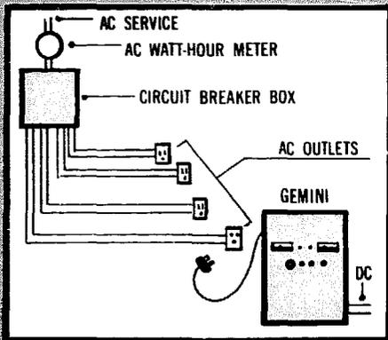
Three phase units can be wired in permanently to the circuit breaker box serving the AC loads or facility in question. For both single phase and three phase applications the Gemini should be isolated on its own circuit and circuit breaker. Power from the DC source is then fed through the Gemini to the circuit breaker box where it is automatically distributed to any AC loads or fed back to the AC source.
