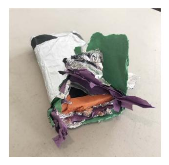
You just made a Faraday shield with three layers of foil alternating with paper. For added security in the future, you can keep adding more layers of foil and paper.
