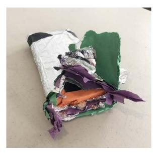
You just made a Faraday shield with three layers of foil alternating with paper. For added security in the future, you can keep adding more layers of foil and paper.
