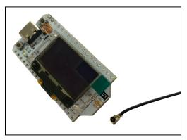
If you're using a Heltec LoRa32, your antenna uses an IPEX-1 connector. The port you'll connect it to is on the front of the device, to the right of the LCD screen.
