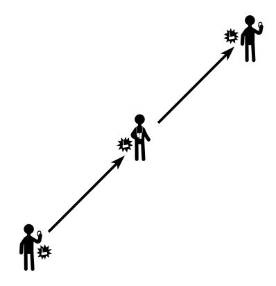
Nodes can also be set up as standalone repeaters that simply route traffic through the network without being connected to a host device. This allows nodes to be operated in an isolated or otherwise fixed position, supplying connection to the greater network for others nearby. This can be an ideal configuration for solar-powered nodes that are elevated for line-of-sight connection, requiring little to no maintenance from the operator.
